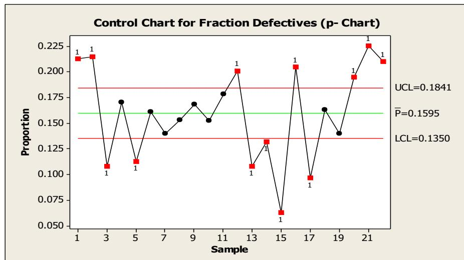
**Conclusion:** From the above  $p$ -chart, we see that the fraction defectives corresponding to the sample numbers 1, 2, 3, 5, 12, 13, 14, 15, 16, 17, 20, 21, 22 fall outside the control limits. So we conclude that the process is out of control.
